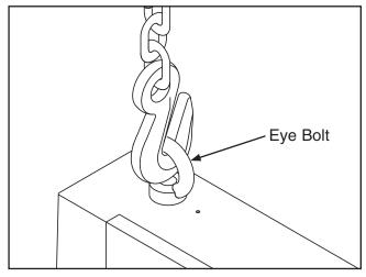
Figure 13. Lifting the bandsaw.
